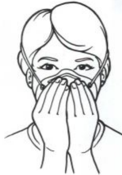
Figure 3 Positive pressure user seal check – Disposable filtering facepiece respirator
