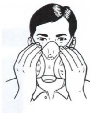
Figure 2 Positive pressure fit check
