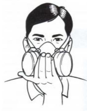
Figure 2 Positive pressure fit check
